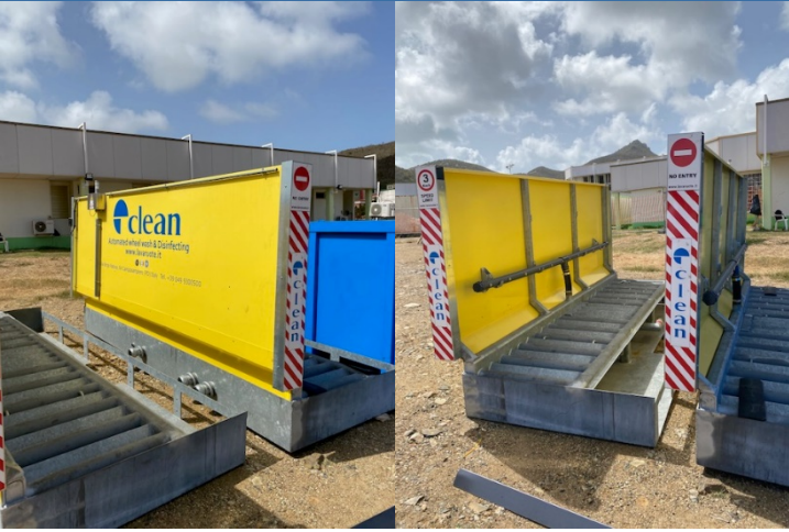
Wheel washing station
